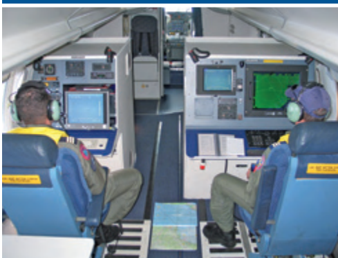
View from the CATO seat in a Dash-8 aircraft of the radar and communication stations
