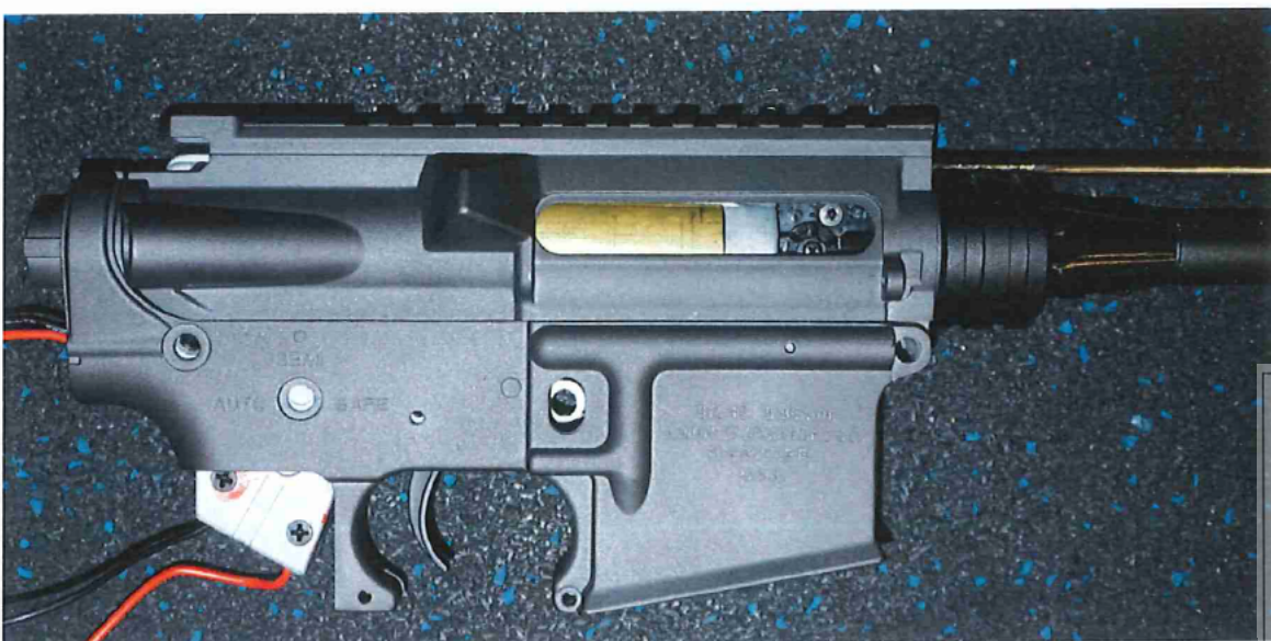
4.6 – Right hand side of one of the upper and lower receivers from Q0115360 fitted with a gear box and barrel from a Lancer Tactical soft air rifle.
