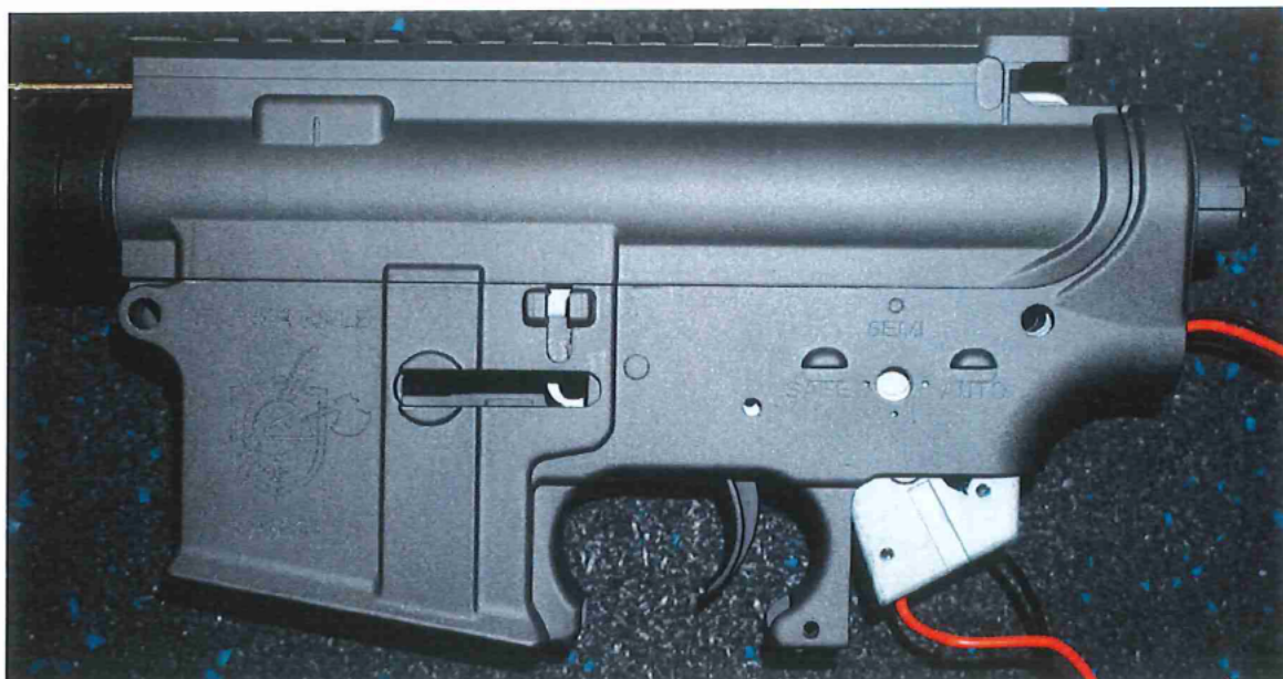
4.7 – Left hand side of one of the upper and lower receivers from Q0115360 fitted with a gear box and barrel from a Lancer Tactical soft air rifle.
