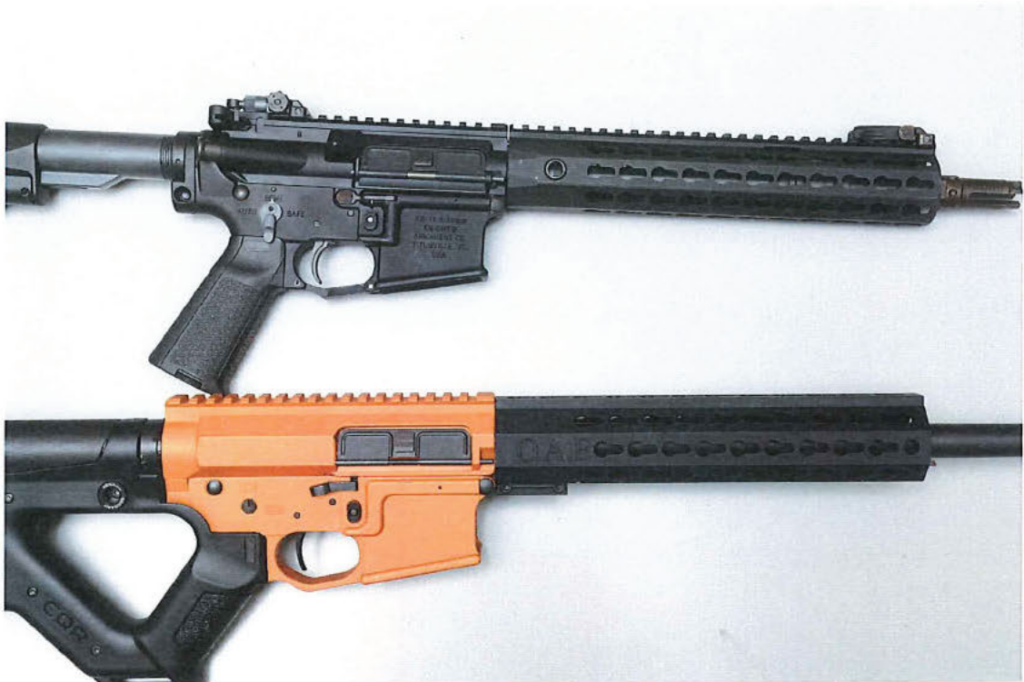
4.5 Photograph of right hand side of Riverman brand, O.A.F. model rifle (below) and Stoner CQB Mod 2 rifle (above) with ejection port cover closed.
