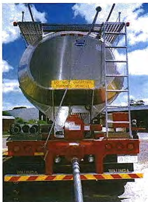
(above right) Rear view showing pneumatic (blower) discharge line, elevated walkways with fold-away guardrails, rear-dump discharge outlet with cover closed.
