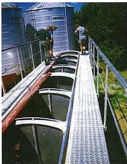
(above left) Top view showing wide-access multi-compartment design. Note - walkways with full-height fold-away guardrails.
