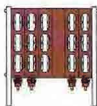
4-way switchboard with busbar sectionaliser unit.
