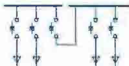
4-way switchboard with busbar sectionaliser unit.
