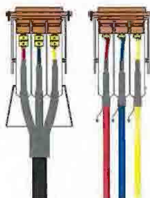
Transformer connection for Magnefix type MF.
