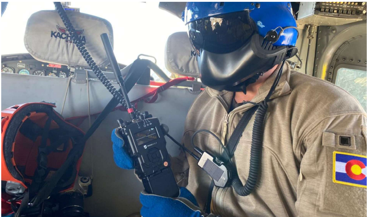
Image: DroneShield's RfPatrol Mk2 drone detection system used by helicopter operators for enhanced situational awareness
